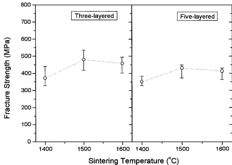
Figure 2 Fracture strength measured by diametral compression disc test for three- and five-layer composites as a function of sintering temperature.
