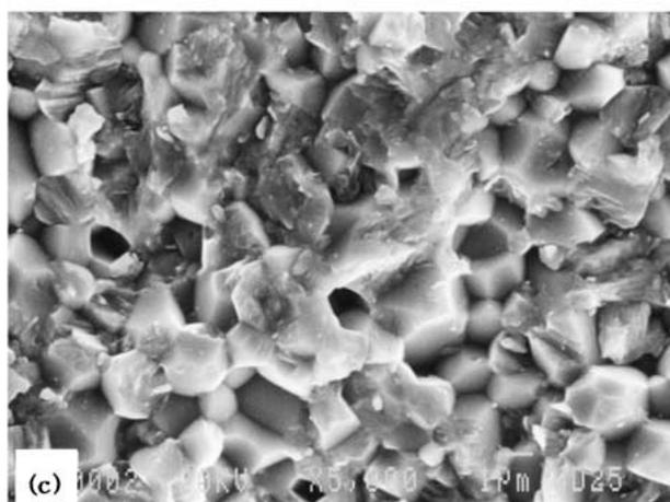
Figure 5 Fracture surfaces of (a) layer 'A' in three-layer composite indented at 49 N load, after sintering at 1500°C, (b) layer 'C' in five-layer indented at 294 N load, after sintering at 1500°C and (c) layer 'B' in five-layer indented at 196 N load, after sintering at 1600°C.
