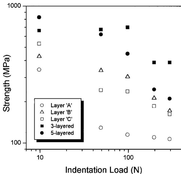
Figure 4 Bend strength of monolithic and layered materials sintered at 1500°C after indentation at different loads.
