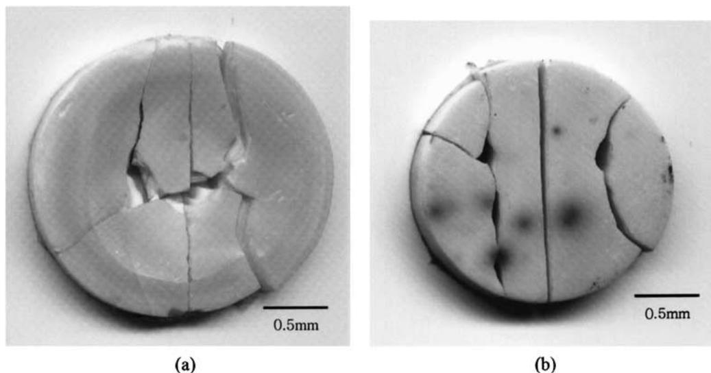
Figure 3 Fractures observed in (a) five-layer composite sintered at 1400°C and (b) three-layer composite sintered at 1500°C.
