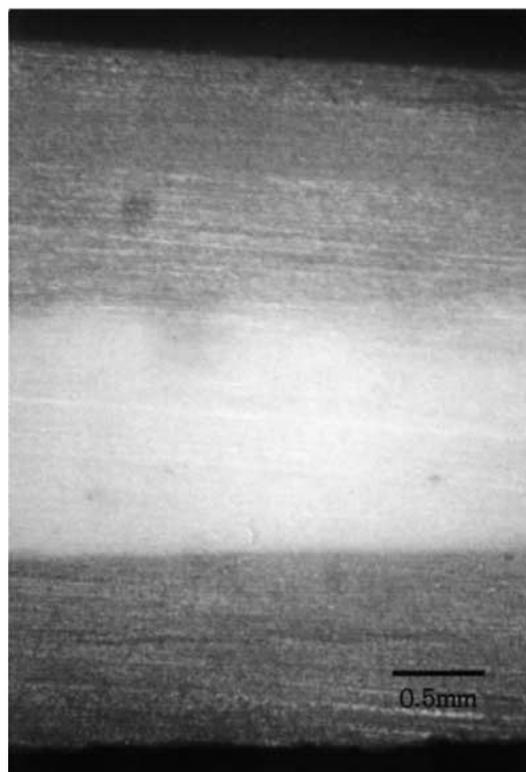
Figure 1 Optical micrograph showing three-layer structure of composite sintered at 1500°C for 2 h.
